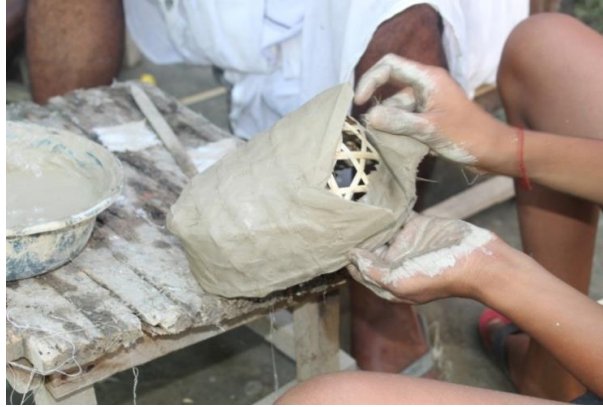
Figure 14 Cover the bamboo frame by potter clay with the help of cotton cloth Source by author
